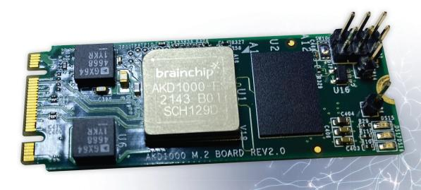
**Fig.5** The BrainChip AKD1000 evaluation board contains the Unified Convolutional Neuromorphic chip. BrainChip also provides a free tool called MetaTF<sup>™</sup> that integrates seamlessly with popular frameworks to allow developers to build and deploy AI smoothly. More information is available on BrainChip's Website. <u>https://brainchip.com/akida-enablement-platforms/</u>
